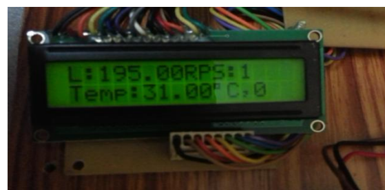
Fig 10 LCD Display showing Level,RPS & Temperature
