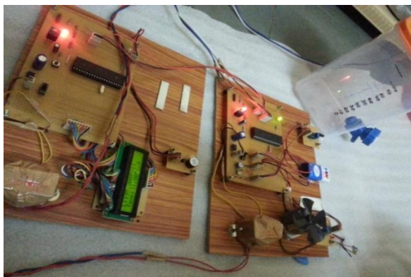
Fig 7 Prototype of the vehicle monitoring system using CAN protocol
